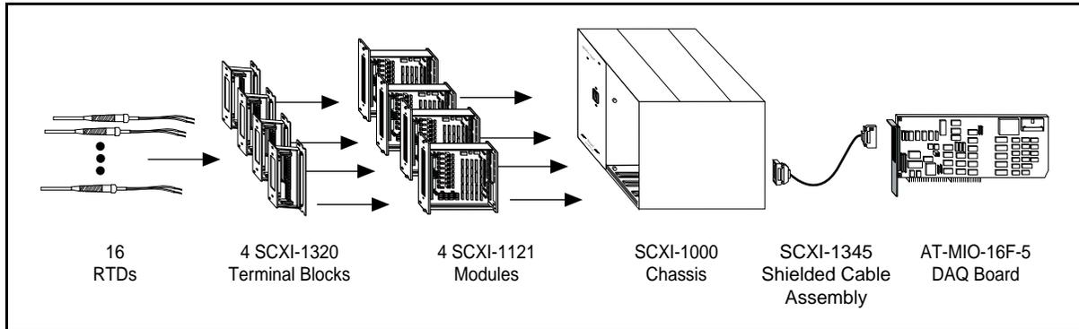
Figure 5. SCXI System for Monitoring 16 RTDs
