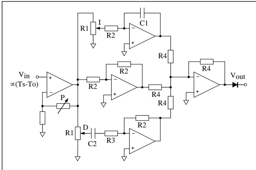
**Figure 6.** Circuit for home-brew PID control.
