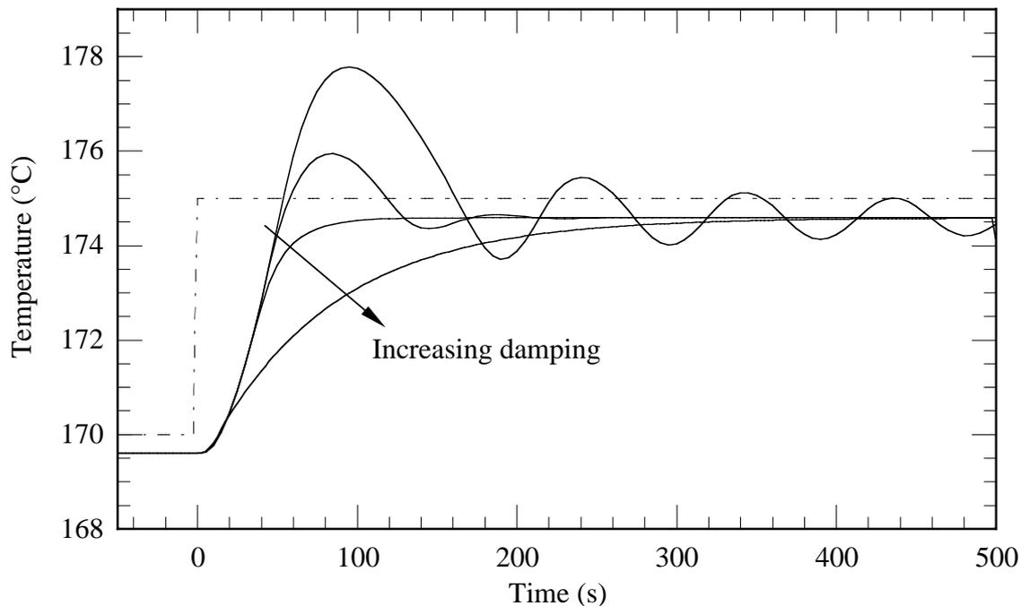
**Figure 4.** Proportional + derivative control. The proportional gain is kept constant as the damping  $\mu$  is increased.
