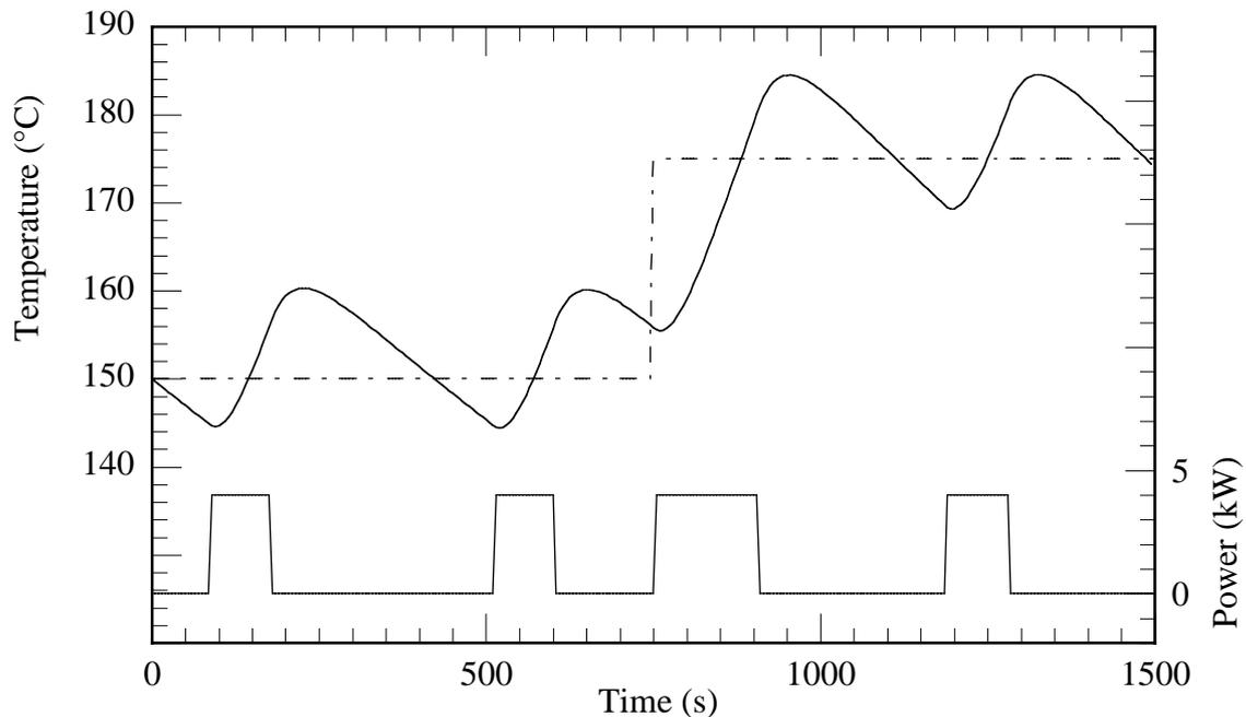
**Figure 2.** The oven ( $T_o$ , solid) and set-point ( $T_s$ , dashed) temperatures using an on-off controller with hysteresis band  $\Delta=10^\circ\text{C}$ .
