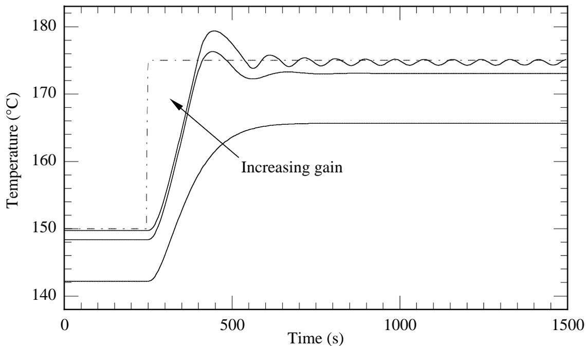
**Figure 3.** Proportional control. (The power is limited to  $\dot{Q}_{\max} = 4$  kW during the early part of the transient.)
