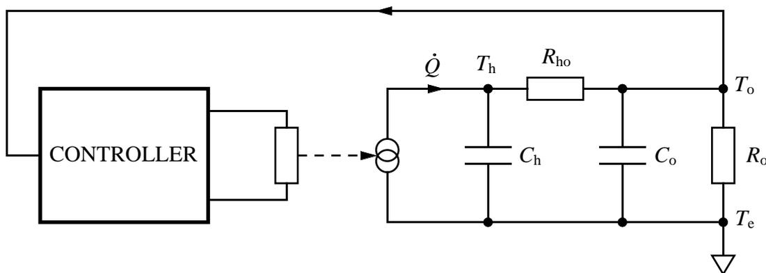
**Figure 1.** Thermal model of oven and controller.
