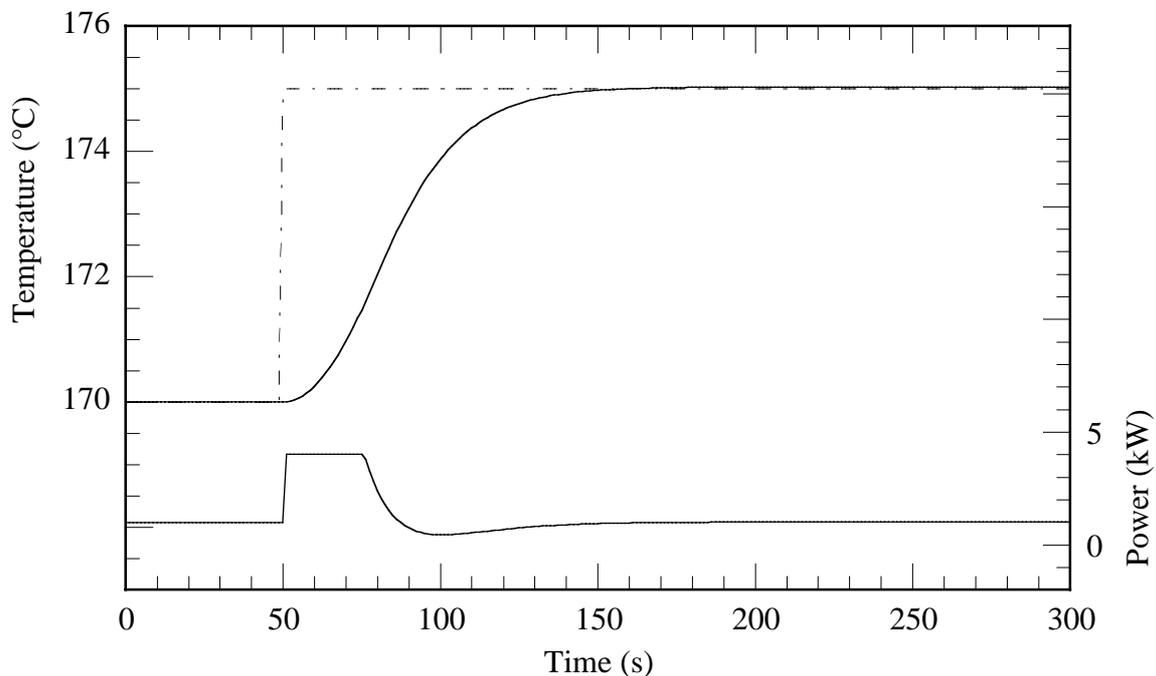
**Figure 5.** PID control. Adding the integral term has eliminated the steady state error. The slight undershoot in the power suggests that there is scope for further tweaking.
